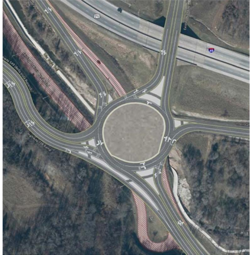
*Interim Modified Connector (Roundabout) will be used at Highway 71B, Highway 71 and I-49 Interchange in Bentonville, AR.*
