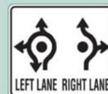
The lane choice sign shows drivers which lanes are used for right turns, straight through travel, left turns and U-turns.
